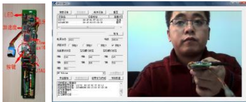
Figure 2. Controller Hardware (left subfigure) and Data Collection Software (right subfigure)
